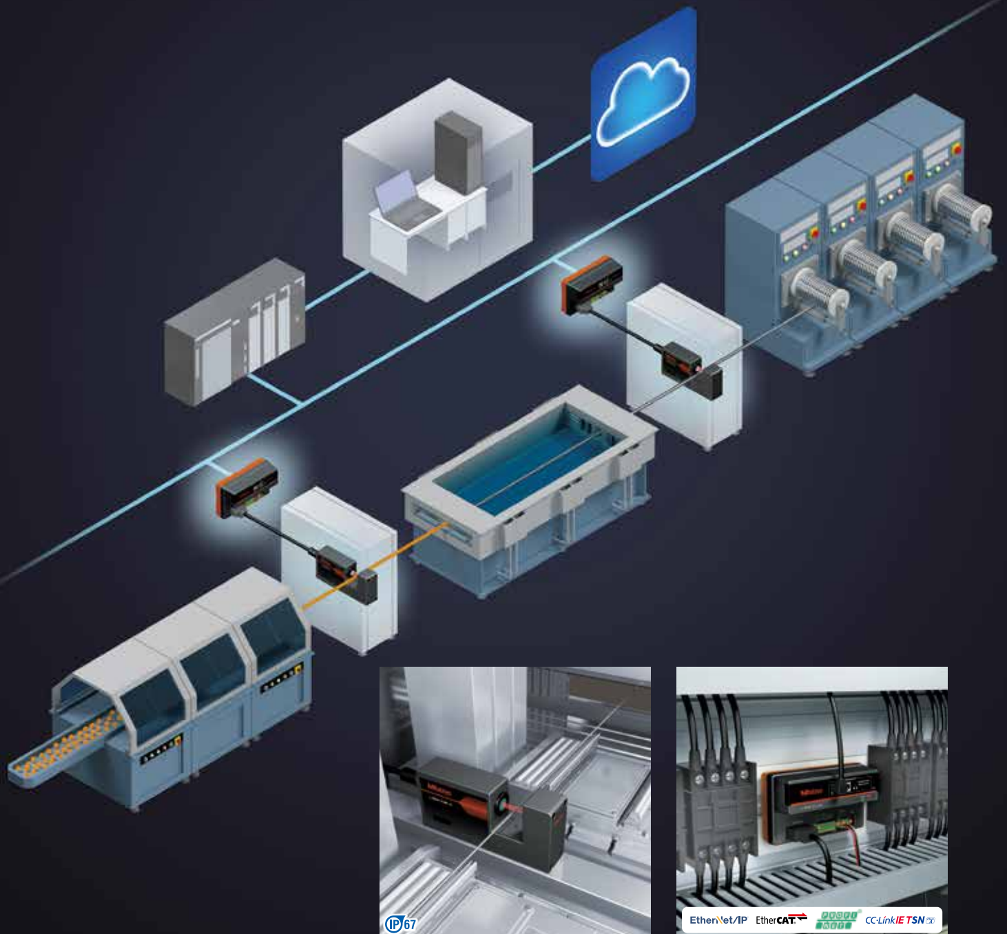
Its thin profile makes it easy to mount on a DIN rail and suitable for installation in a distribution board
