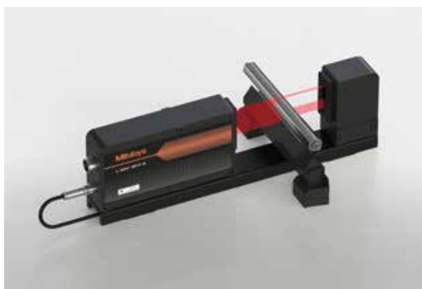
Simultaneous measurement of roller outside diameter and deflection
